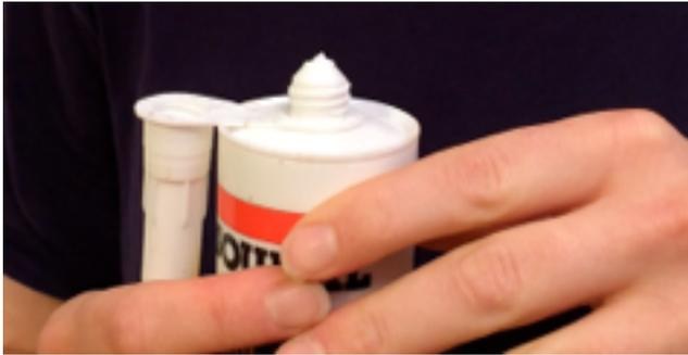
*Trim the domed end off the cartridge using a retractable blade.*
