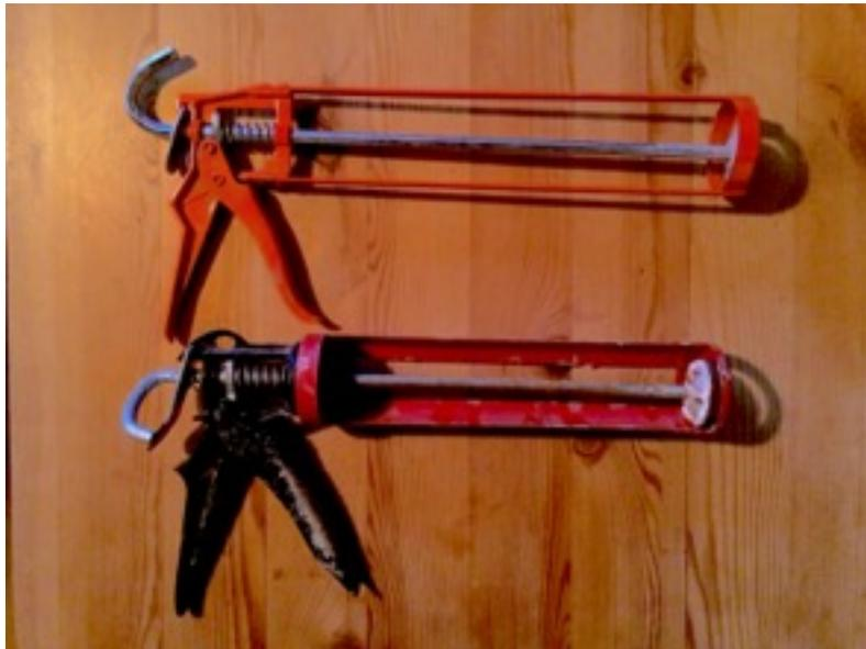
The cartridge gun, also called a sealant/skeleton/mastic gun, is what you need for doing any jobs with sanitary sealant in your bathroom.
